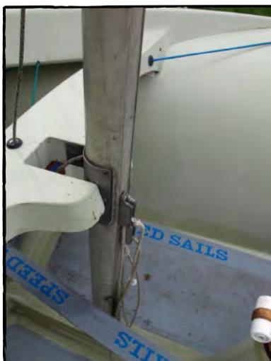
Photo 2, mast and jammers
