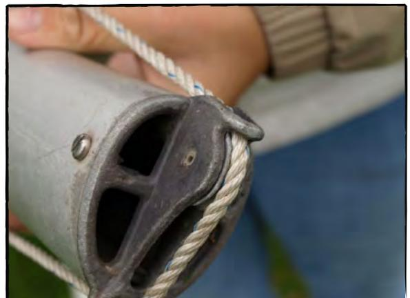
Photo 18, Pass the rope around the boom end
