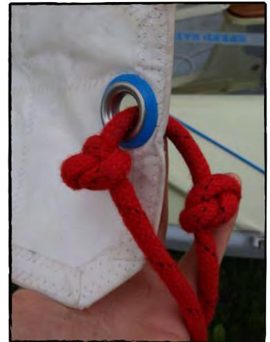
Photo 12, attach the jib sheet
